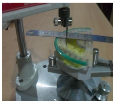
Fig 5: A protector is placed on the cast to maintain parallelism
