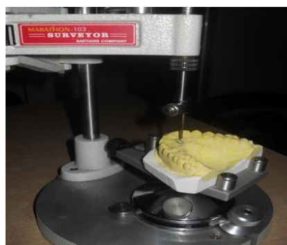
Fig 4: Cast secured on the surveyor
