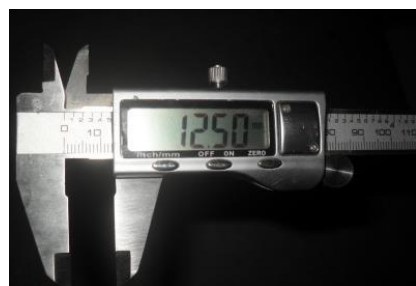
Fig 7: Distance is measured by digital Vernier calipers
